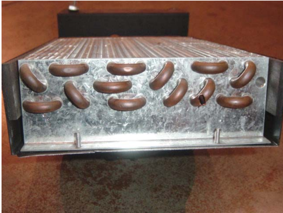
LEAKING UNDER-SEAT HEATING UNIT (10,280 TEST MILES)
