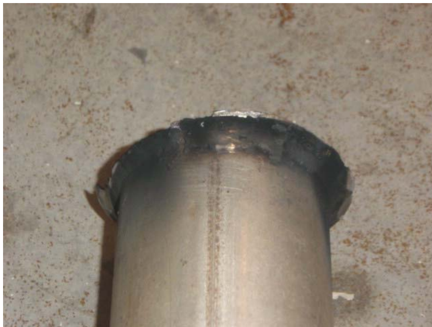
BROKEN FLANGE ON PIPE TO EXHAUST MANIFOLD (1,648 TEST MILES)
