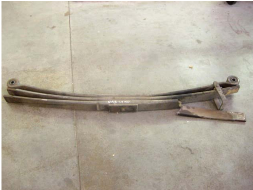
BROKEN RIGHT REAR LEAF SPRING (3,752 TEST MILES)
