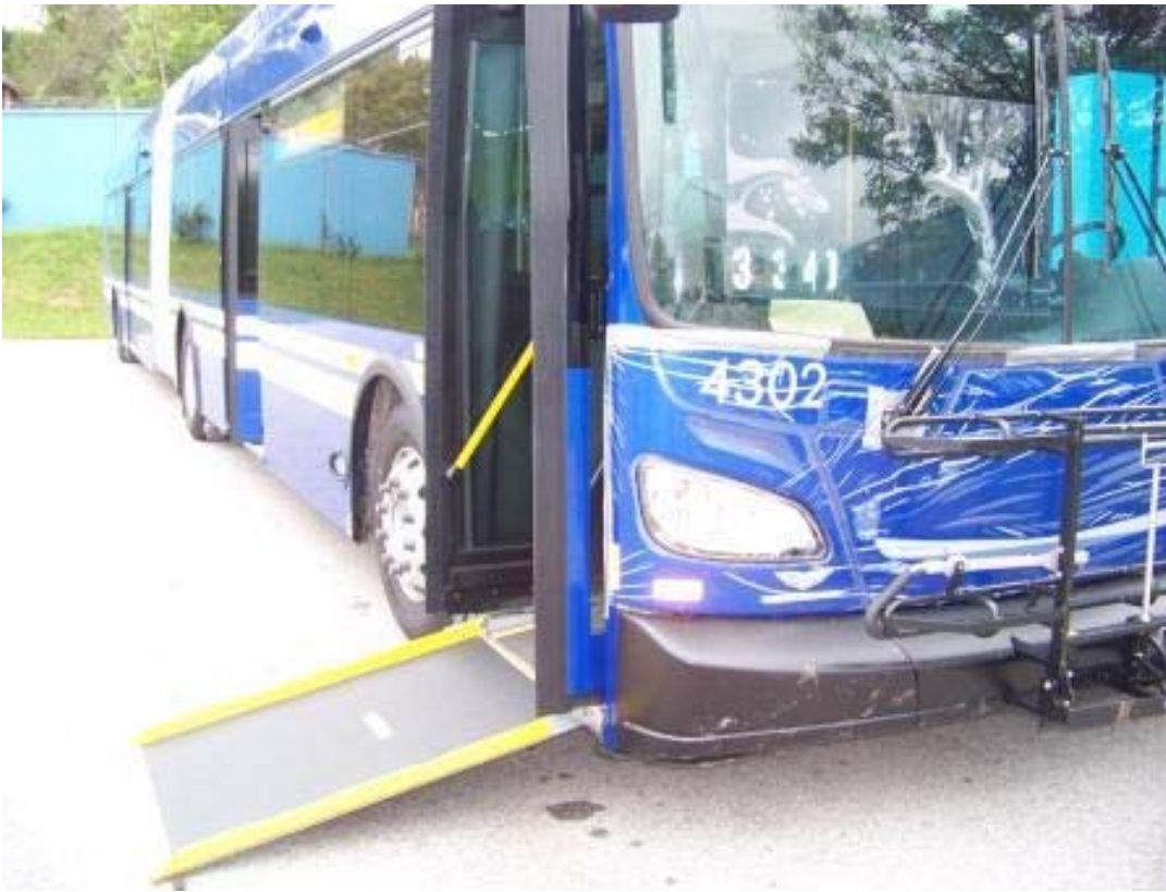
NEW FLYER MODEL XDE60 EQUIPPED WITH A NEW FLYER FOLDOUT HANDICAP RAMP
