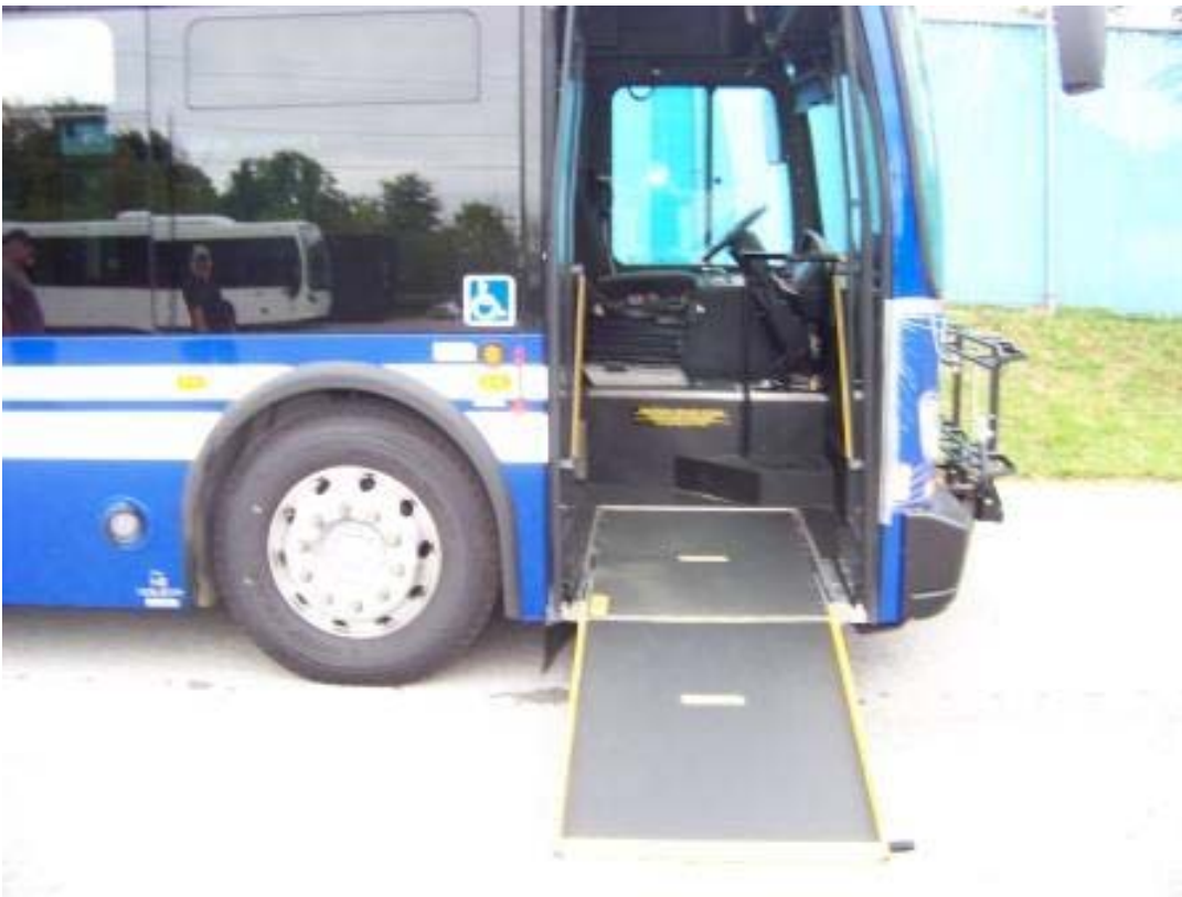
NEW FLYER MODEL XDE60 EQUIPPED WITH A NEW FLYER FOLDOUT HANDICAP RAMP
