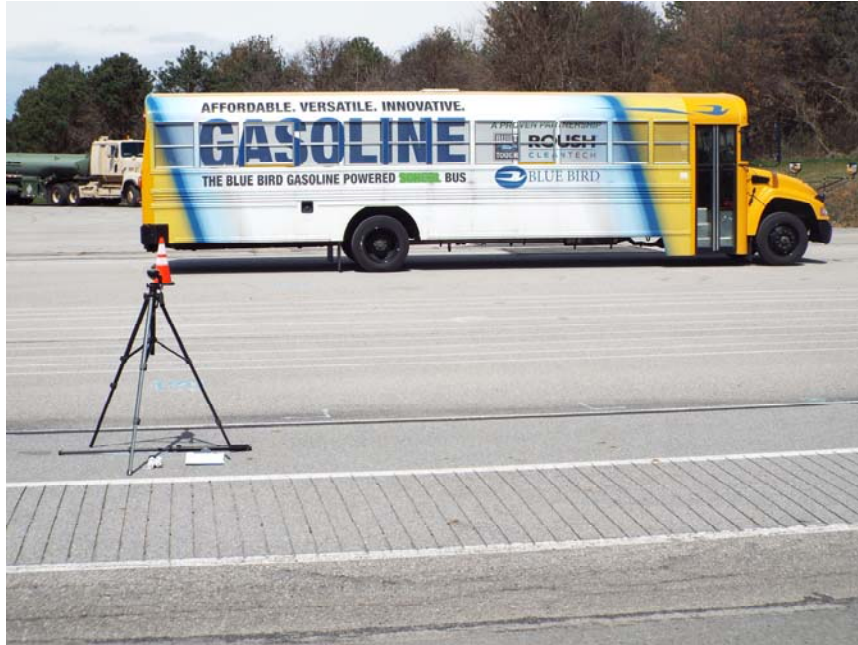
TEST BUS UNDER GOING EXTERIOR NOISE TESTING
