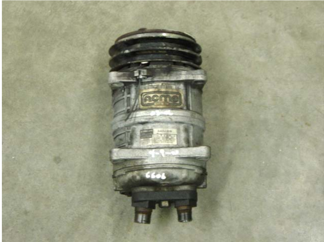
FAILED A/C COMPRESSOR CLUTCH (6,217 TEST MILES)
