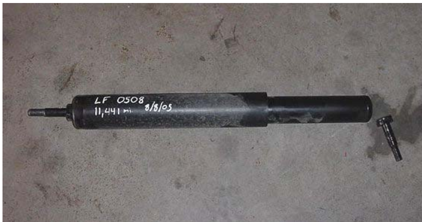
FAILED LEFT FRONT SHOCK (10,436 TEST MILES)
