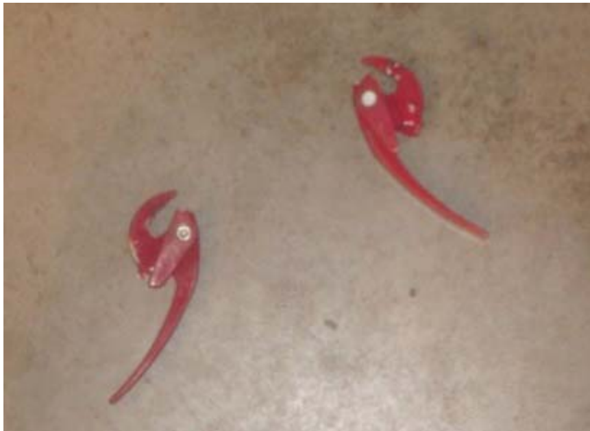
BROKEN WINDOW LATCHES (1,333 TEST MILES)
