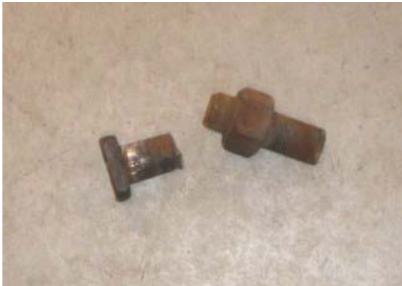
BROKEN BOLT FROM CROSS MEMBER BELOW ENGINE (2,900 TEST MILES)
